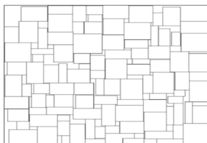
Figure.9. Floorplan of n100 GSRC benchmark with area = 20.0455mm 2 and interconnect length= 19.5489mm.
