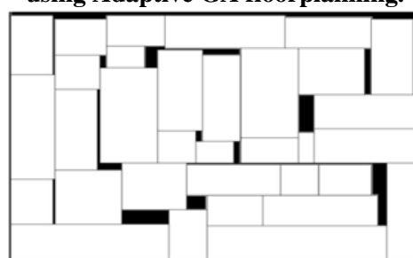
Figure.8. Floorplan of ami33 benchmark with area = 1.21mm 2 and total Interconnect length = 31.33mm
